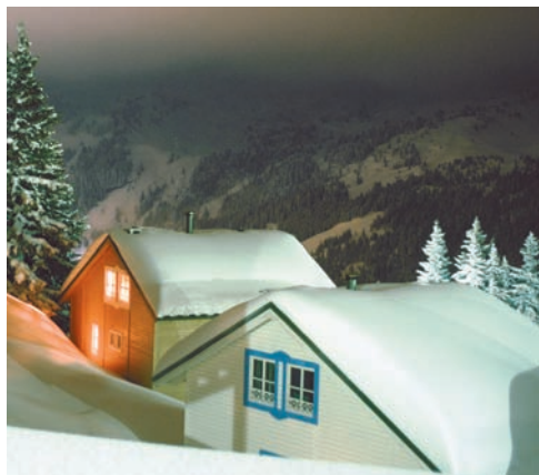
Photo 5.3 The roofs of the buildings shown must be able to support not only the total weight of the snow but also the nonsymmetric distributed loads resulting from drifting of the snow.
