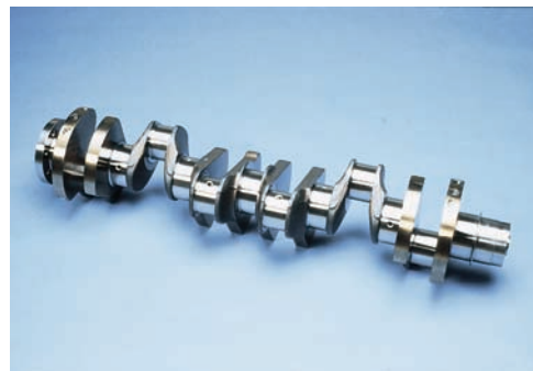
Photo 18.4 The forces exerted by a rotating automobile crankshaft on its bearings are the static and dynamic reactions. The crankshaft can be designed to be dynamically as well as statically balanced.
