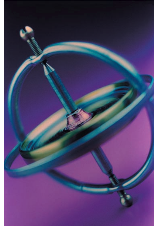
Photo 18.5 A gyroscope can be used for measuring orientation and is capable of maintaining the same absolute direction in space.
