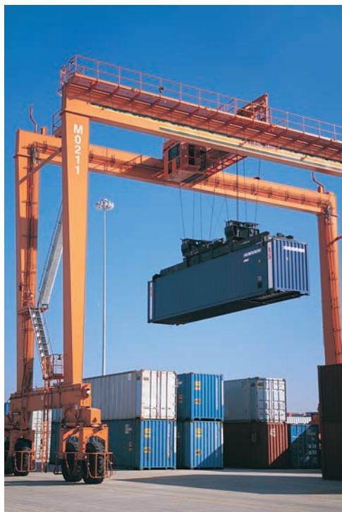
Photo 11.2 Multiple cables and pulleys are used by this shipyard crane.
