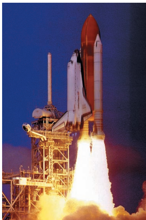
Photo 14.3 As the shuttle's booster rockets are fired, the gas particles they eject provide the thrust required for liftoff.
